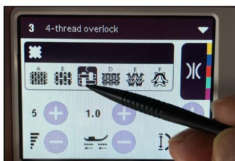
If any fine-tuning of the looper threads is desired, you can use the Precise Thread Control. This patented feature on your AMBER™ Air S|600 allows for fine-tuning the overedge threads for perfect stitch formation along fabric edges.
